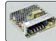
SUR-MW-75W Input(AC) : 85-264V/120-373V Output(DC): 12V/24V Power : 75W Certification: CE, CCC, CB Size : 99*97*30mm Waterproof : Non-waterproof
