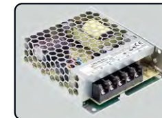
SUR-MW-50W Input(AC) : 85-264V/120-373V Output(DC): 12V/24V Power : 50W Certification: CE, CCC, CB Size : 99*82*30mm Waterproof : Non-waterproof
