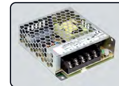
SUR-MW-35W Input(AC) : 85-264V/120-373V Output(DC): 12V/24V Power : 35W Certification: CE, CCC, CB Size : 99*82*30mm Waterproof : Non-waterproof
