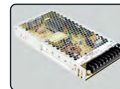
SUR-MW-200W Input(AC) : 90-132V/180-264V Output(DC): 12V/24V Power : 200W Certification: CE, CCC, CB Size : 215*115*30mm Waterproof : Non-waterproof
